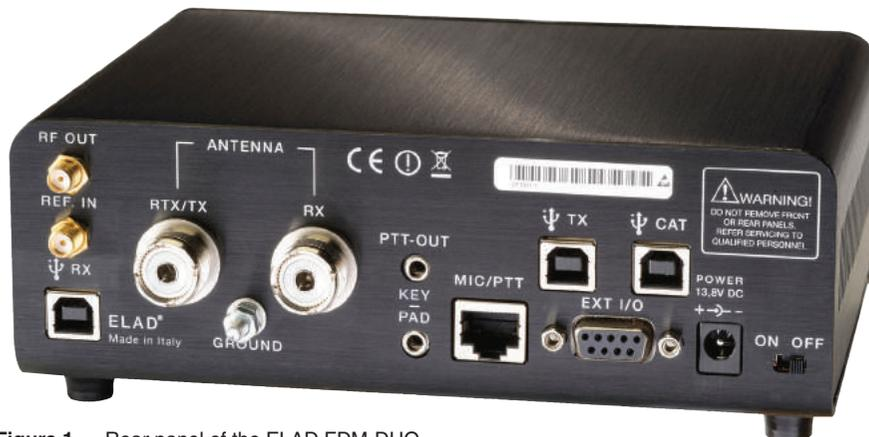
Figure 1 — Rear panel of the ELAD FDM-DUO.
